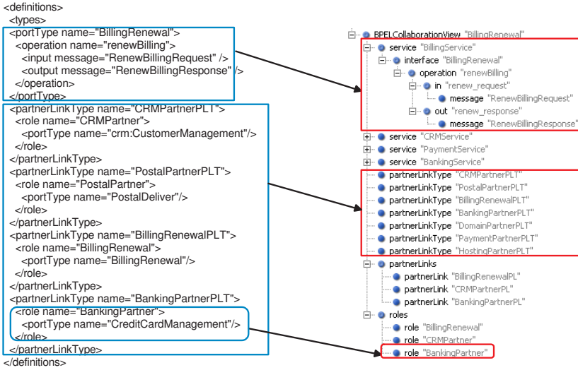
Fig. 6. Mapping the Billing Renewal process (left-hand side) onto the Collaboration View (right-hand side)
